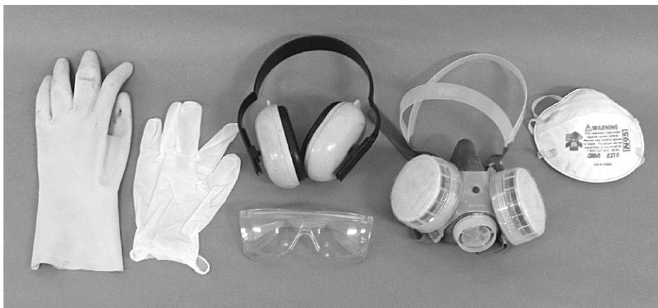
Some safety equipment: rubber and latex gloves, hearing protectors, safety glasses, toxic dust mask, nuisance dust mask.
