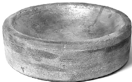
Concrete bowl: cast using the process above. 12" (30 cm) across.
