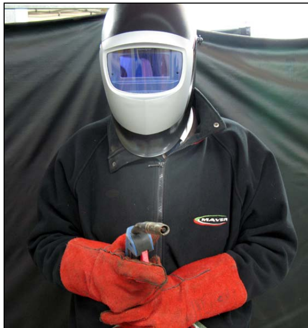
Gloves, auto-darkening helmet and a suitable cotton based jacket are essential to keep safe
