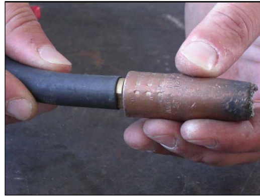
6. Replace the welding cup
