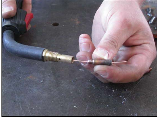
3. Unscrew the bad welding tip
