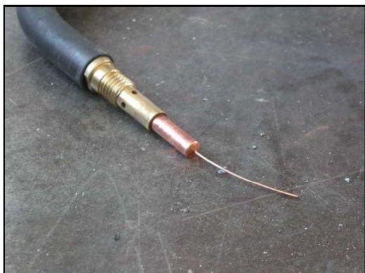
5. Screw the new tip on
