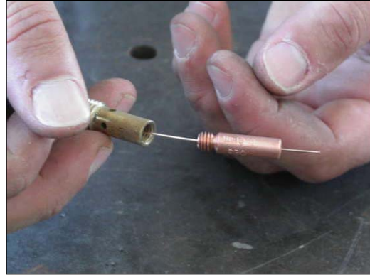
4. Slide a new tip into place.
