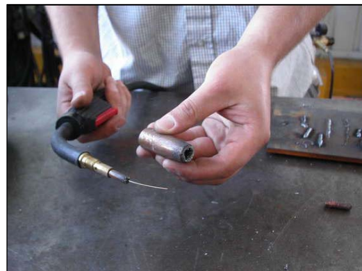
2. Unscrew the welding shield cup.
