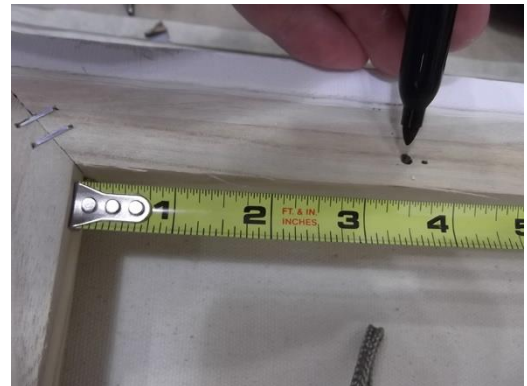
Figure 1. Marking the D-ring hole location
