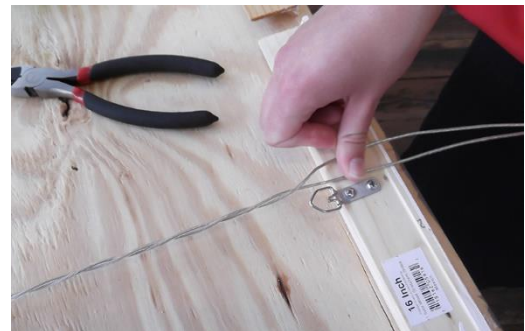
Figure 18. Wire is twisted too tightly
