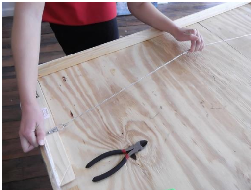
Figure 21. Stretching the twisted wires
