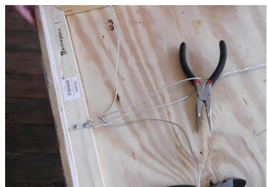
Figure 24. Holding the wires apart with plier weight
