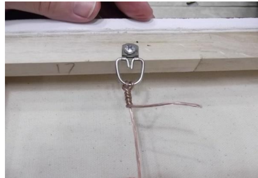
Figure 6. Finishing the wrap—about 3/4 inch long
