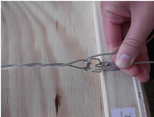
Figure 19. Starting the lock stitch on each end
